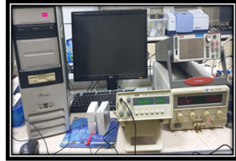
Figure 6: I-V characteristic test system
